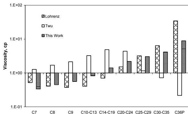
Fig. 7 Comparison of component viscosities with different critical volume estimation methods (after regression) – Black Oil
